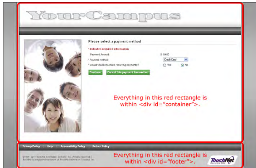
The main DIV on uPay web pages has an ID of "container." The footer DIV has an ID of "footer."
