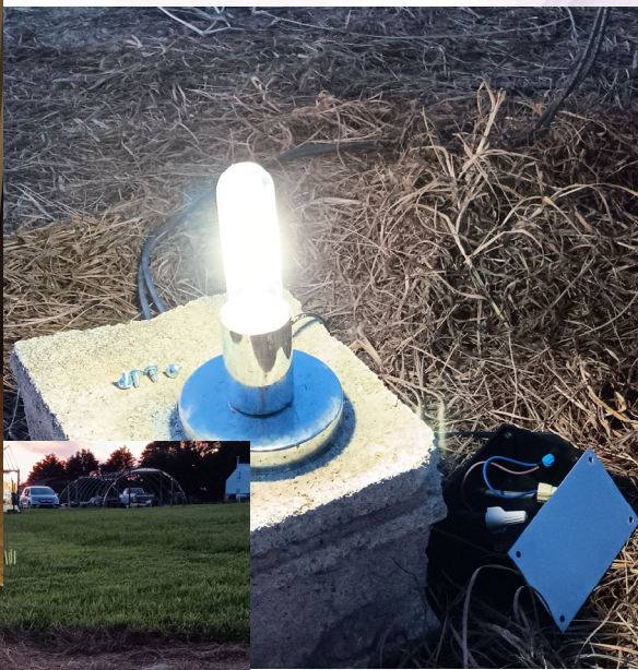
Dr. Charles Van Neste lamps powered by sensors in the soil.
